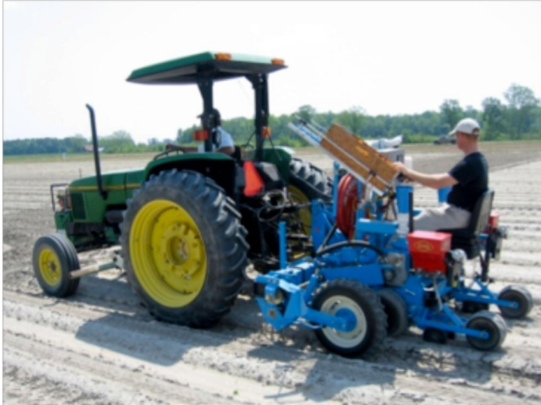
Figure 1. Planting sorghum with a NG Plus 3 Monosem two-row precision vacuum planter in plots of two- 40 ft. rows on 36-inch centers.
