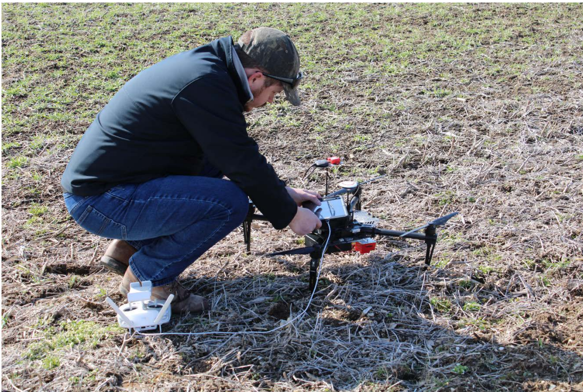
Figure 4: Dr. Joseph Oakes prepares the UAV that carries the NDVI and NDRE sensors for flight over wheat plots to measure tiller densities at GS 25.
